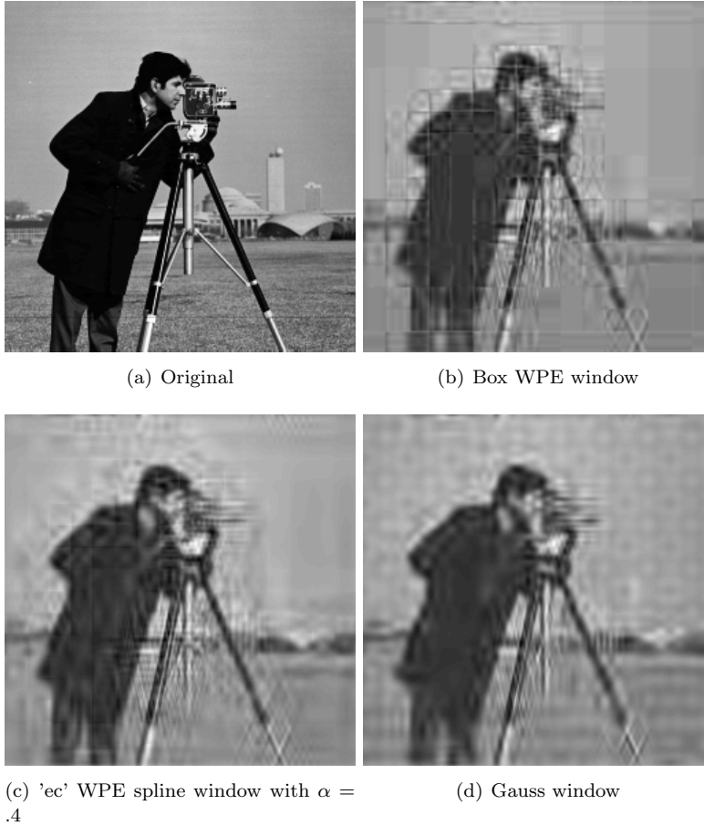
Fig. 5. The figure shows a test done on a standard test image, the Cameraman. The image in the upper left corner is the original 256x256 greyscale image. The other 3 images have been compressed using a 2D Wilson basis with M = 16 channels and different window functions as specified below each image. The specified window was used for synthesis and the corresponding canonical dual window was used for analysis. The 1% largest coefficients have been kept, and all other coefficients set to zero.
