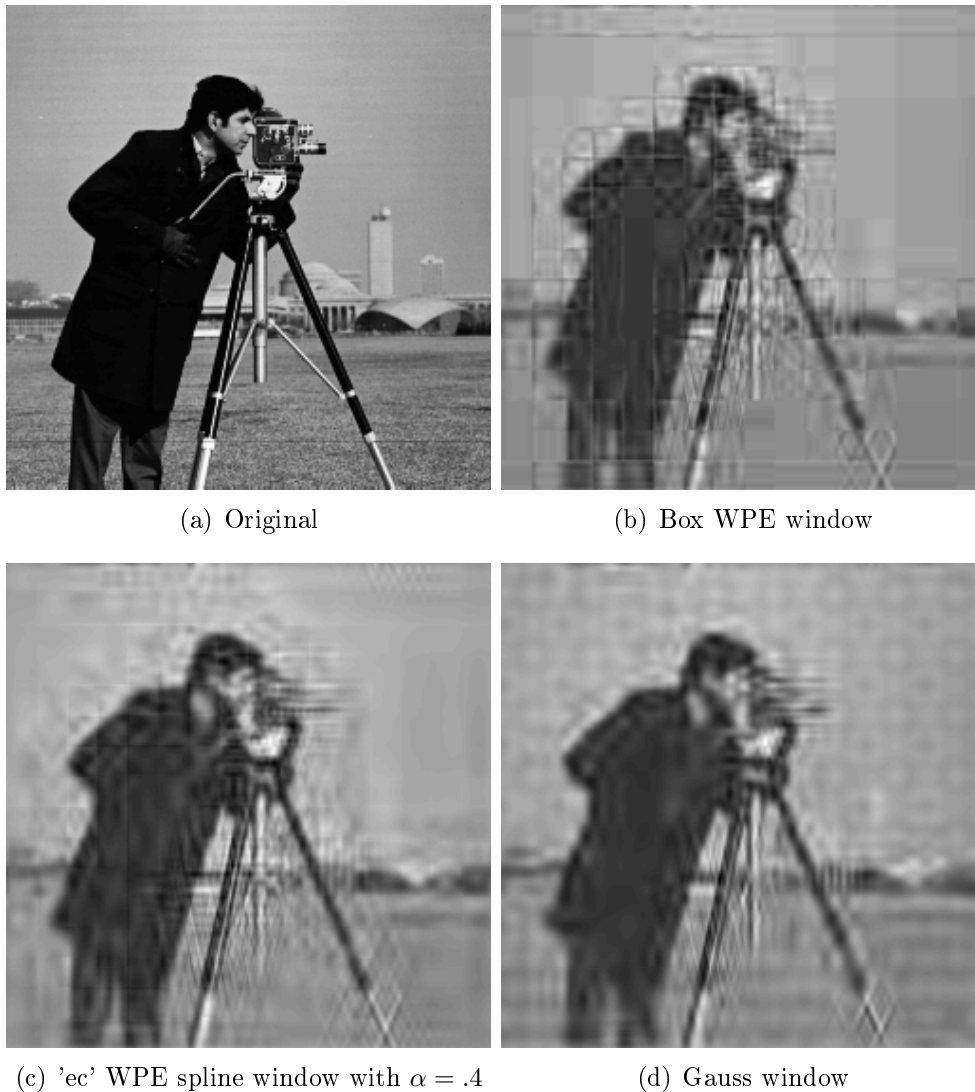
Figure 3.5: The figure shows a test done on a standard test image, the Cameraman. The image in the upper left corner is the original 256x256 greyscale image. The other 3 images have been compressed using a 2D Wilson basis with M = 16 channels and different window functions as specified below each image. The specified window was used for synthesis and the corresponding canonical dual window was used for analysis. The 1% largest coefficients have been kept, and all other coefficients set to zero.
