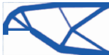
Fig. 3.4. A refined version of the design shown in Fig. 3.3, using a resolution of 12,800 "pixels" – this demands more computer power, resulting in a more well-defined design.
