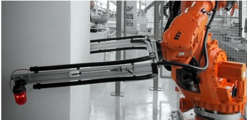
FIGURE 1. Robotic Hot Wire cutting in Odense, Denmark.
