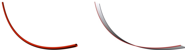
FIGURE 8. Left: A cylindrical rod can cut in any direction that is close to perpendicular to the tangent of the curve. Right: A flat (ribbon) blade design (with its hot edge indicated in red) moves well only in the directions given by the flat extension of the blade past the hot edge itself.
