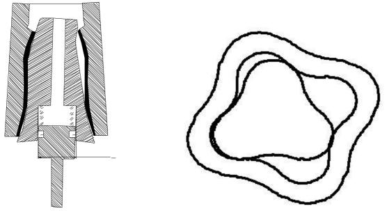
\* For n-teeth running inside n+1 teeth: make an expression for as well internal as well as external element with different eccentricities.
