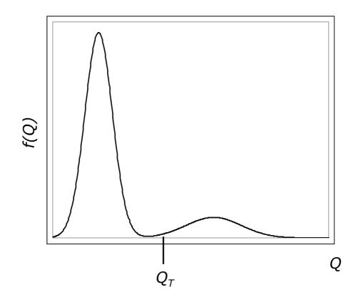
Figure 1: Typical distribution of decay rates. Most components have decay rates lower than the threshold, but some have larger, and should therefore be discarded by the control procedure.
