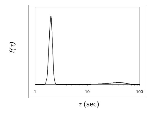
Figure 2: Typical distribution of the dynamic response, which is actually the delay time after the control procedure is started on a component until the signal from its Q begins to build up (see Fig. 3). With only a couple of seconds available, some malfunctioning components will actually not be caught in our present control procedure.
