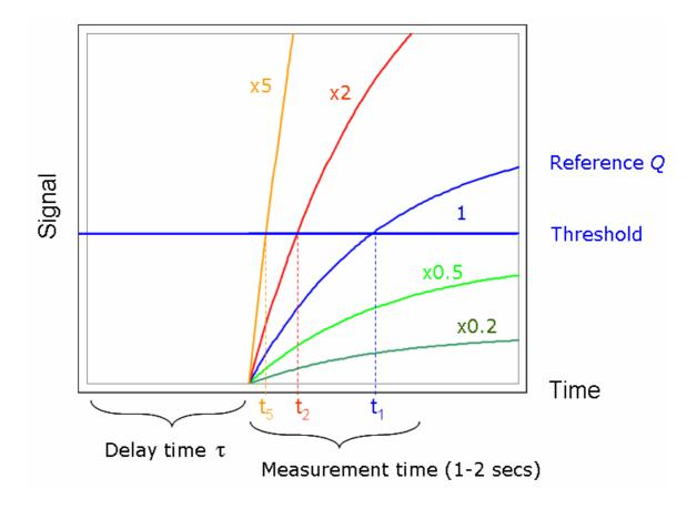
Figure 3: The temporal development of the signal after the control procedure is started. After a certain delay time, the signal starts to build up exponentially. The magnitude of the signal is then recorded during a short measurement period time (1–2 secs), often before it has reached its steady state value. If it is above that of a calibrated reference which has  $Q = Q_T$ , like those denoted x2 and x5 in the figure, the control procedure makes sure that the component in question is discarded.
